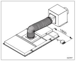
3) The motor unit can be freely positioned. Connection to the appliance is via the exhaust ducting and the connection cable.
